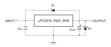
CIN:  $0.1~\mu\text{F}$  or higher. Set this value according to the length of the line between the regulator and INPUT pin. Be sure to connect CIN to prevent parasitic oscillation. Use of a film capacitor or other capacitor with excellent voltage and temperature characteristics is recommended. If using a laminated ceramic capacitor, it is necessary to ensure that CIN is  $0.1~\mu\text{F}$  or higher for the voltage and temperature range to be used.
