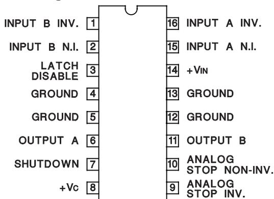
Note: All four ground pins must be connected to a common ground.
