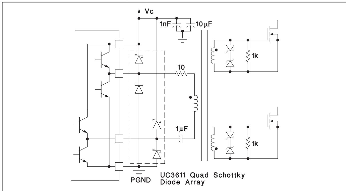
Figure 4. Transformer coupled push-pull MOSFET drive circuit.
