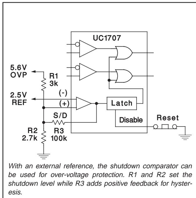
Figure 6. Over-voltage protection.
