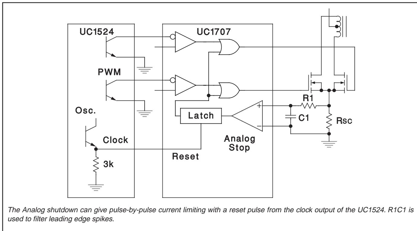
The Analog shutdown can give pulse-by-pulse current limiting with a reset pulse from the clock output of the UC1524. R1C1 is used to filter leading edge spikes.
