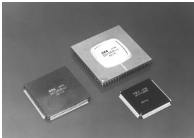
Figure 1. Sample CMOS-8 Packages
