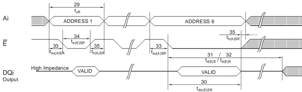
u:  $\bar{W}$  must be HIGH when  $\bar{E}$  is LOW during the address sequence in order to initiate a nonvolatile cycle.  $\bar{G}$  may be either HIGH or LOW throughout. Addresses 1 through 6 are found in the mode selection table. Address 6 determines whether the U635H256 performs a STORE or RECALL.
