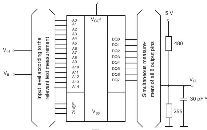
w: In measurement of  $t_{d15}$ -times and  $t_{en}$ -times the capacitance is 5 pF.
