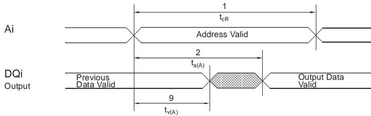
Read Cycle 2:  $\bar{G}$ -,  $\bar{E}$ -controlled (during Read cycle:  $\bar{W} = V_{IH}$ )<sup>g</sup>
