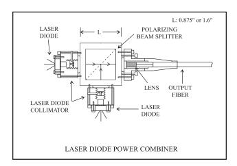
style systems are best suited for applications where the output coupler is used with a multimode fiber. If a receptacle style combiner is used with a singlemode fiber, then the user may have to adjust the alignment to maximize coupling efficiency. Receptacle style systems with better repeatability are available, but at the expense of lower coupling efficiencies.
