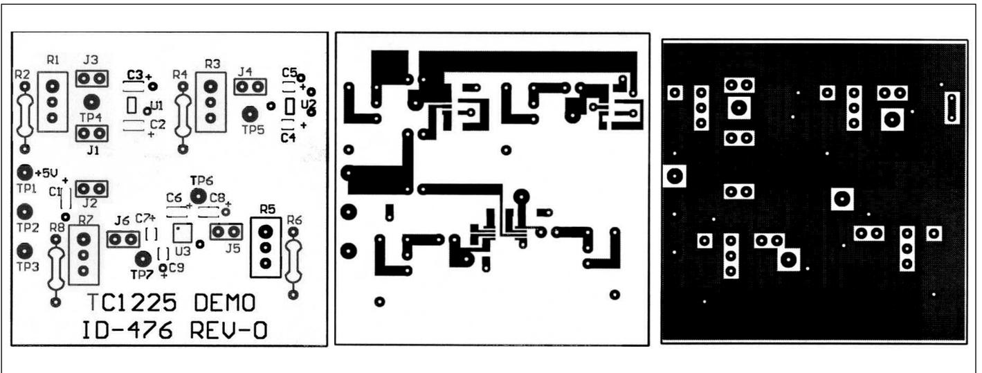
Figure 4. TC1225 DEMO Card Assembly Drawing and Artwork
