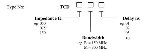
Example Part No: TCD075B02 is a 75  $\Omega$ , 150 MHz, 2 ns delay line. Maximum allowable product of Impedance ( $\Omega$ ) x Delay (ns) is 500 in package DR00165A (eg 050 x 10 = 500). Please contact factory regarding increased impedance/delay products.
