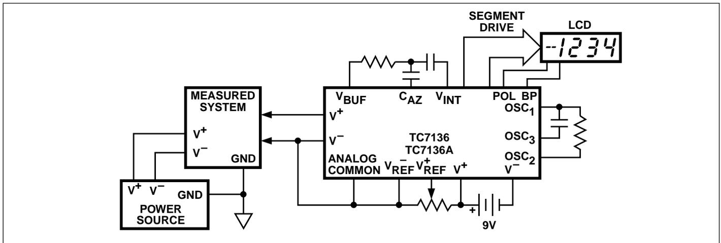
Figure 7. Common-Mode Voltage Removed in Battery Operation With  $V_{IN} = \text{Analog Common}$
