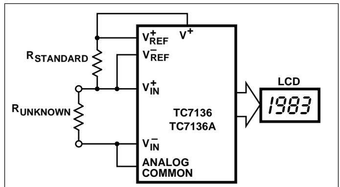
Figure 12. Low Parts Count Ratiometric Resistance Measurement
