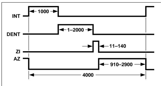
Figure 4. Conversion Timing During Normal Operation
