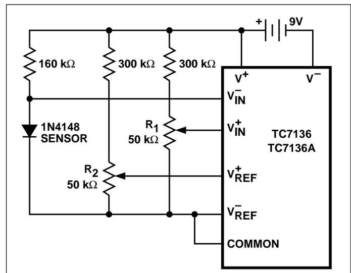
Figure 13. Temperature Sensor
