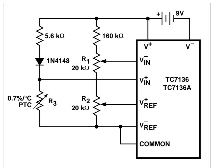
Figure 14. Positive Temperature Coefficient Resistor Temperature Sensor
