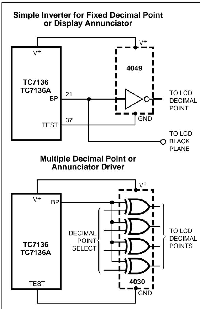
Figure 11. Decimal Point and Annunciator Drives
