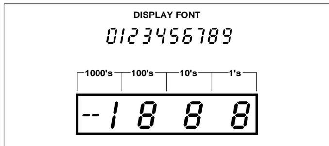
Figure 6. Display FONT and Segment Assignment
