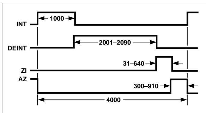
Figure 5. Conversion Timing During Overrange Operation
