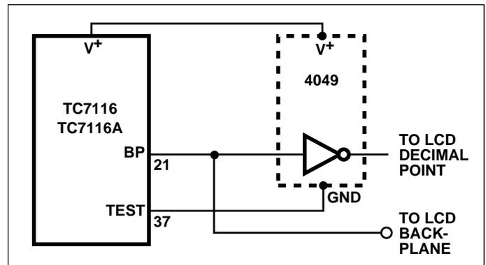
Figure 5. Simple Inverter for Fixed Decimal Point
