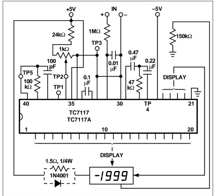
Figure 18. Diode or Resistor Limits Package Power Dissipation
