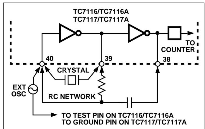
Figure 7. Clock Circuits
