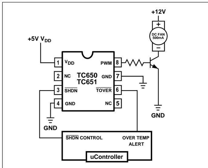
The TC650/651 are integrated temperature sensors and brushless DC fan speed controllers. The TC650/651 measure their junction temperature and control the speed of the fan based on that temperature, making them especially suited for applications in modern electronic equipment.
