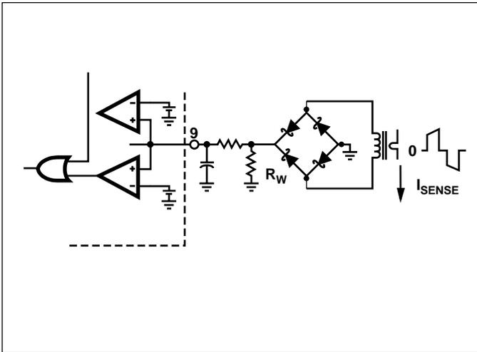
Figure 10. Primary or Secondary Side Current Sensing
