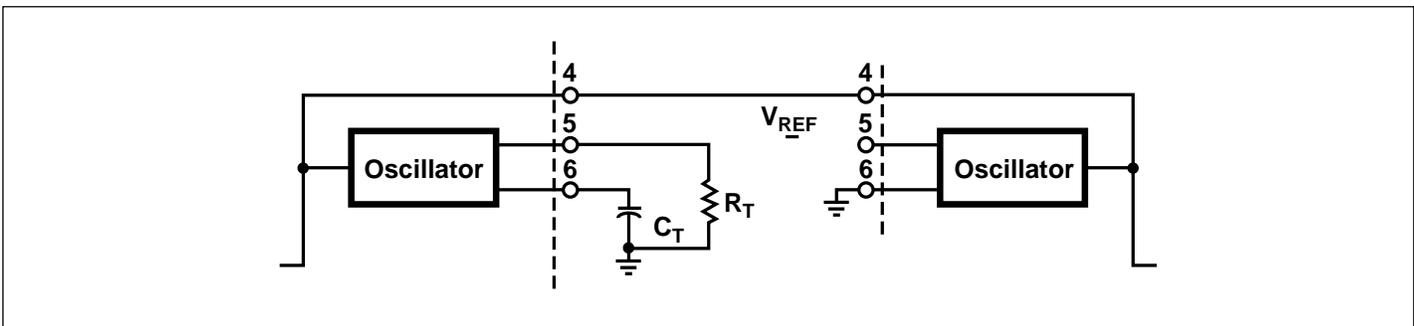
Figure 13. Current Mode Master/Slave Operation Over Short Distances
