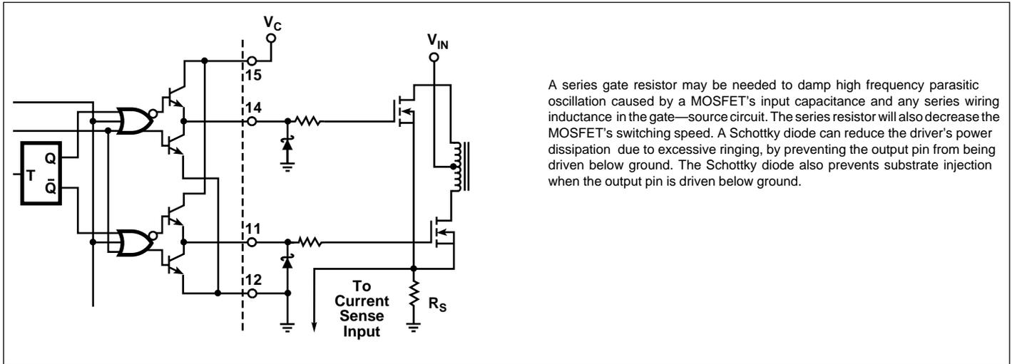
Figure 18. MOSFET Parasitic Oscillations
