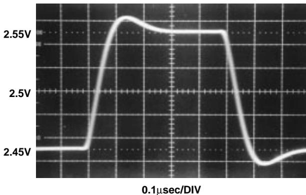
Figure 27. Error Amp Large Signal Transient Response
