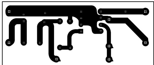
Figure 22. PC Board Layout Copper Side
