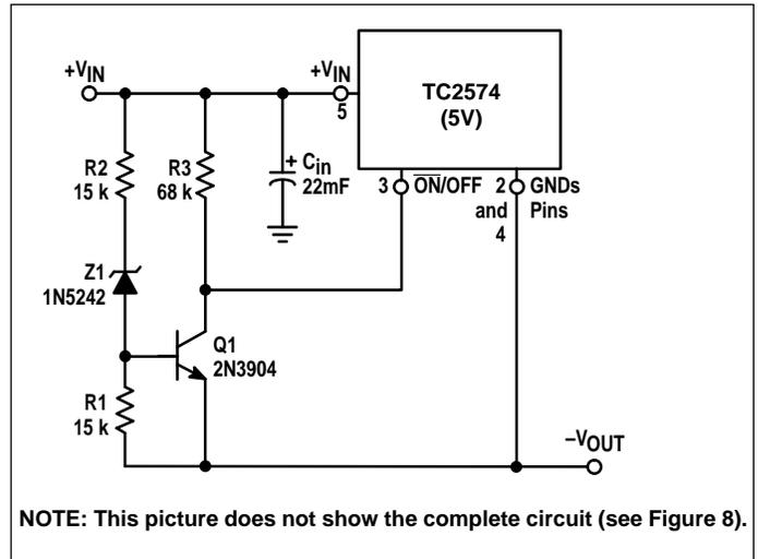
Figure 15. Undervoltage Lockout Circuit for Buck-Boost Converter
