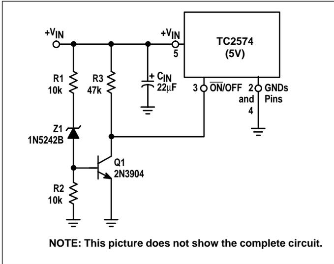
Figure 14. Undervoltage Lockout Circuit for Buck Converter
