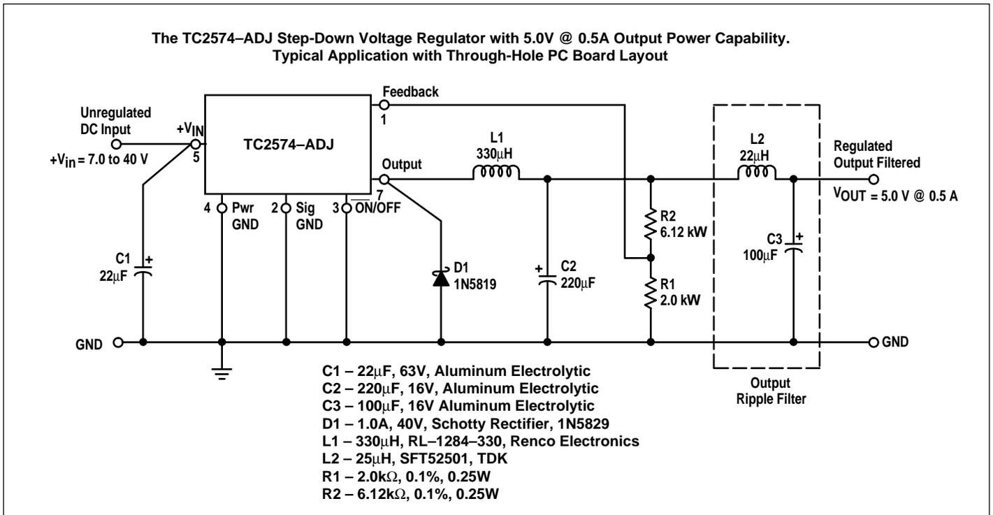
Figure 20. Schematic Diagram of the 5.0V @ 0.5A Step-Down Converter Using the TC2574-ADJ
