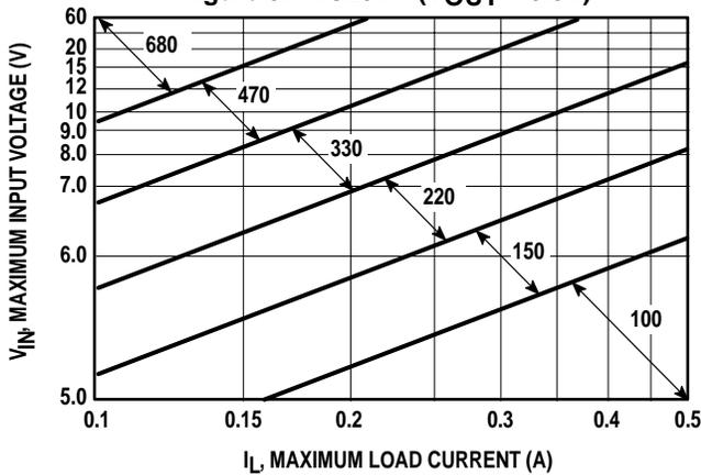
Figure 38. TC2574 ( $V_{\text{OUT}} = 5.0\text{V}$ )
