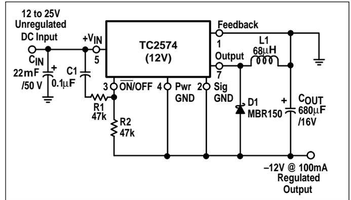
Figure 9. Inverting Buck-Boost Regulator with Delayed Startup
