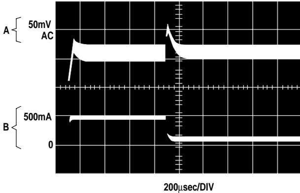
A: Output Pin Voltage 50V/DIV, AC Coupled
