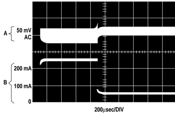
A: Output Pin Voltage 50V/DIV, AC Coupled
