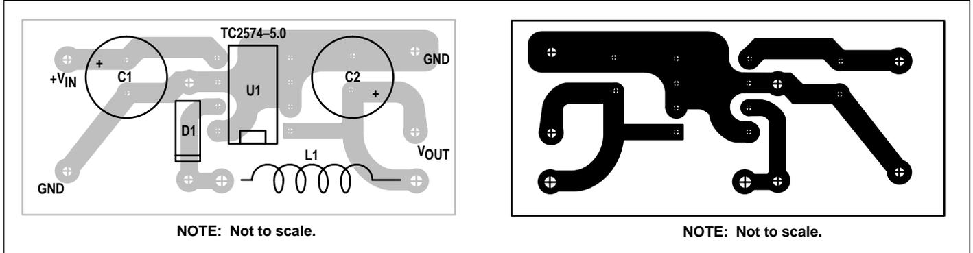
Figure 18. PC Board Layout Component Side
