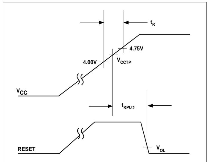
Figure 3. Timing Diagram: Power Up (TC1274)
