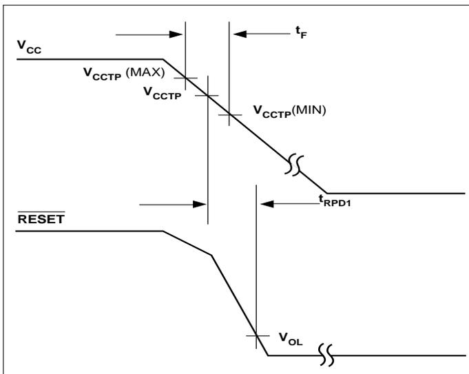
Figure 2. Timing Diagram: Power Down (TC1272, TC1273)
