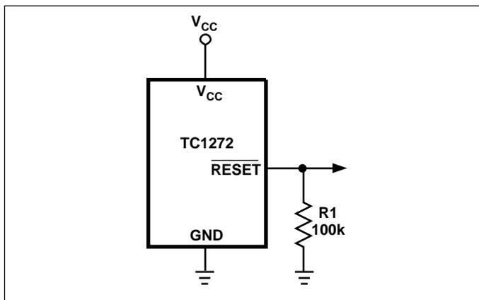
Figure 6. Ensuring  $\overline{\text{RESET}}$  Valid to  $V_{CC} = 0V$
