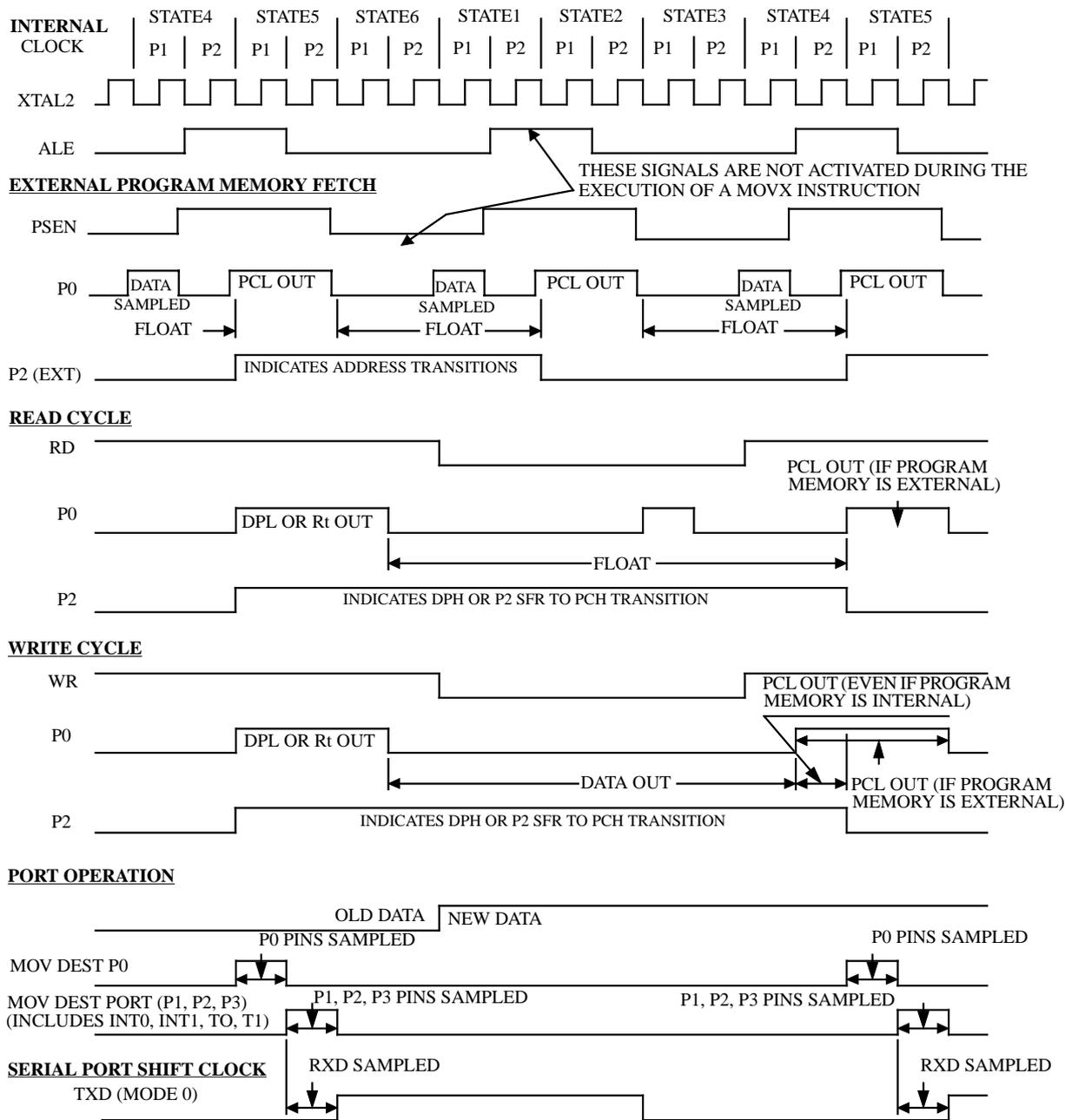
Figure 26. Clock Waveforms
