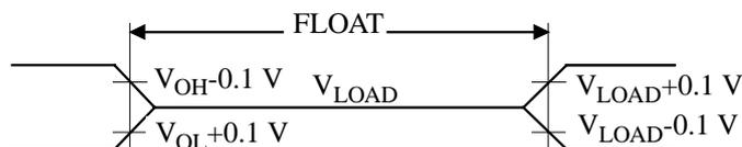
Figure 25. Float Waveforms
