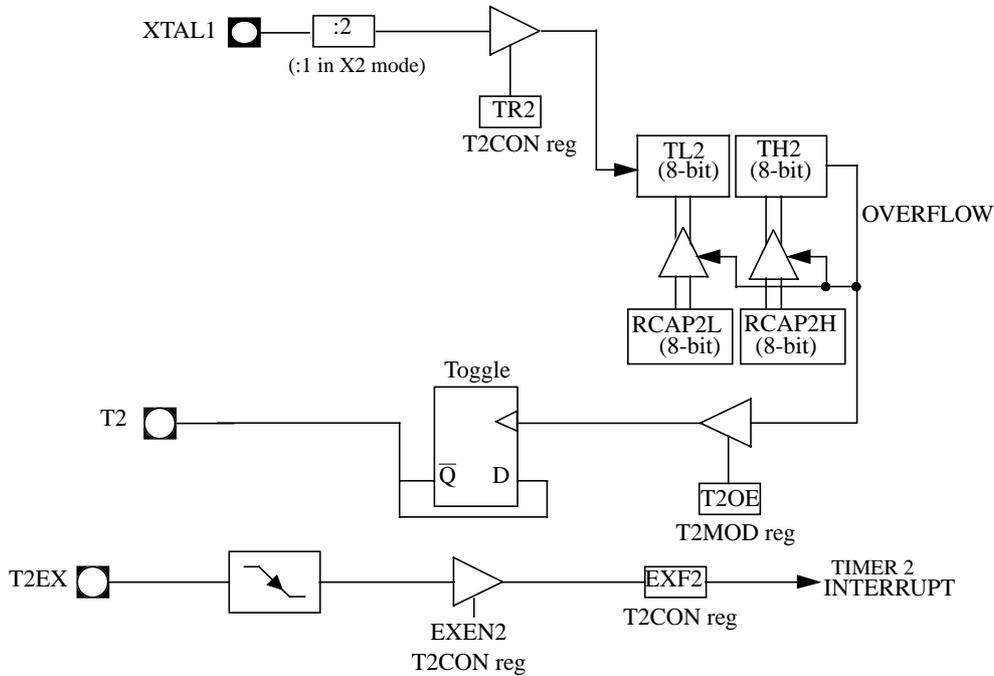
**Figure 5. Clock-Out Mode  $C/\overline{T2} = 0$**
