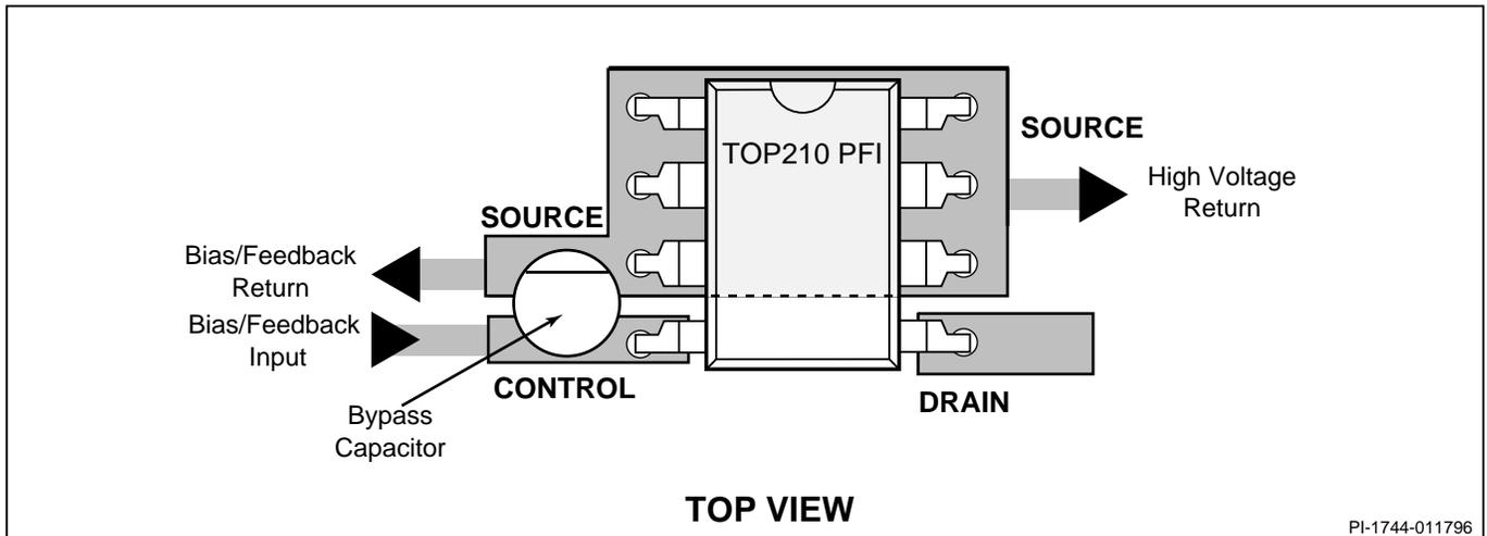
Figure 9. Recommended PC Layout for the TOP209/210.
