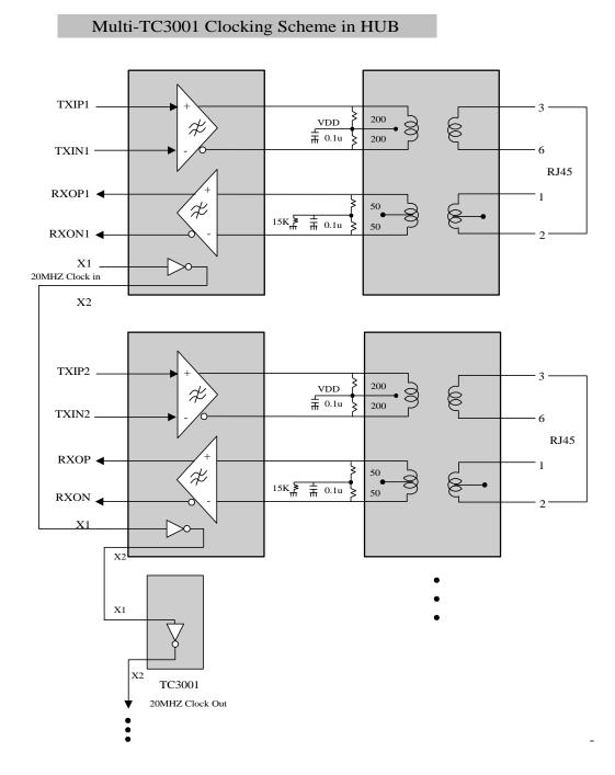
Each TC3001 is connected in series through X1 in and X2 out to next one. This scheme enables the 20MHZ clock to "See" only one CMOS loading. The relative phases between TC3001's are not important. This clock is used for internal precision delay reference only.
