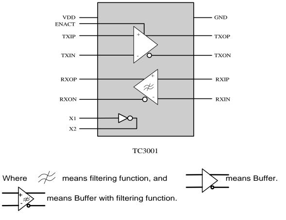
The transmitter converts digital Manchester encoded data from third party twisted pair interface controller to the twisted pair cable. The circuit provides pre-distorted and filtered waveforms so that the outputs are made to appear as if it had passed through 5-7th order external passive filter, thereby only a isolation pulse transformer is needed.
