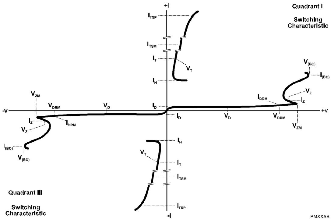
Figure 1. VOLTAGE-CURRENT CHARACTERISTIC FOR TERMINALS A AND B
