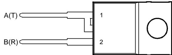
Pin 1 is in electrical contact with the mounting base.
