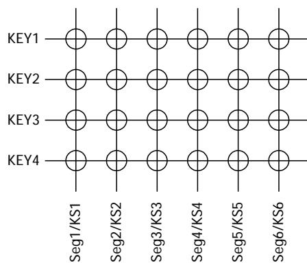
The data of each Key is stored as illustrated below, and is read by a read command, starting from the least significant bit.
