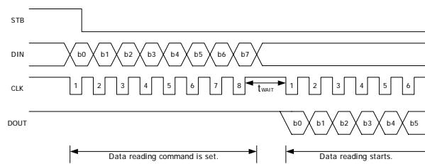
Because the  $D_{OUT}$  pin is an N-ch open-drain output pin, be sure to connect an external pull-up resistor to this pin (1k $\Omega$  to 10 k $\Omega$ ).
