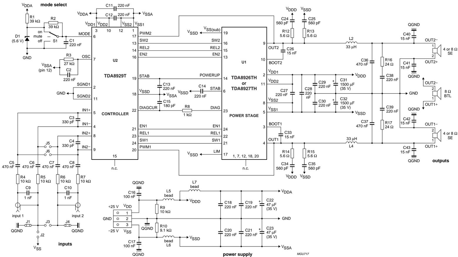
Resistor R1 value  $\leq \frac{V_{DD(min)} - 5.6 V}{100 \mu A} \Omega$ .
