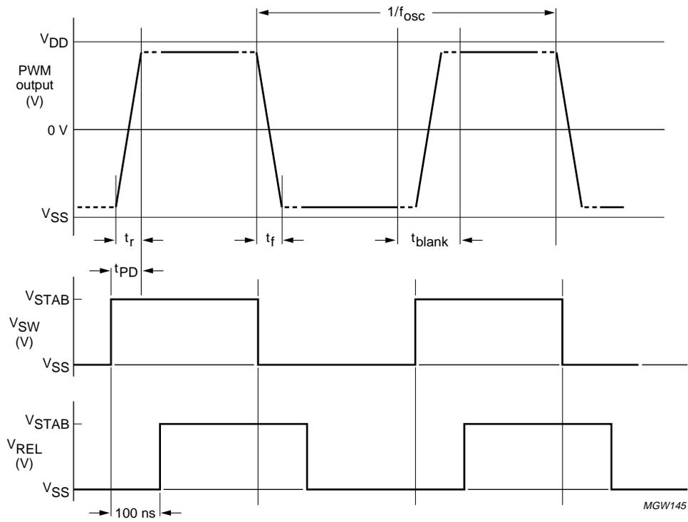
Fig.5 Timing diagram PWM output, switch and release signals.
