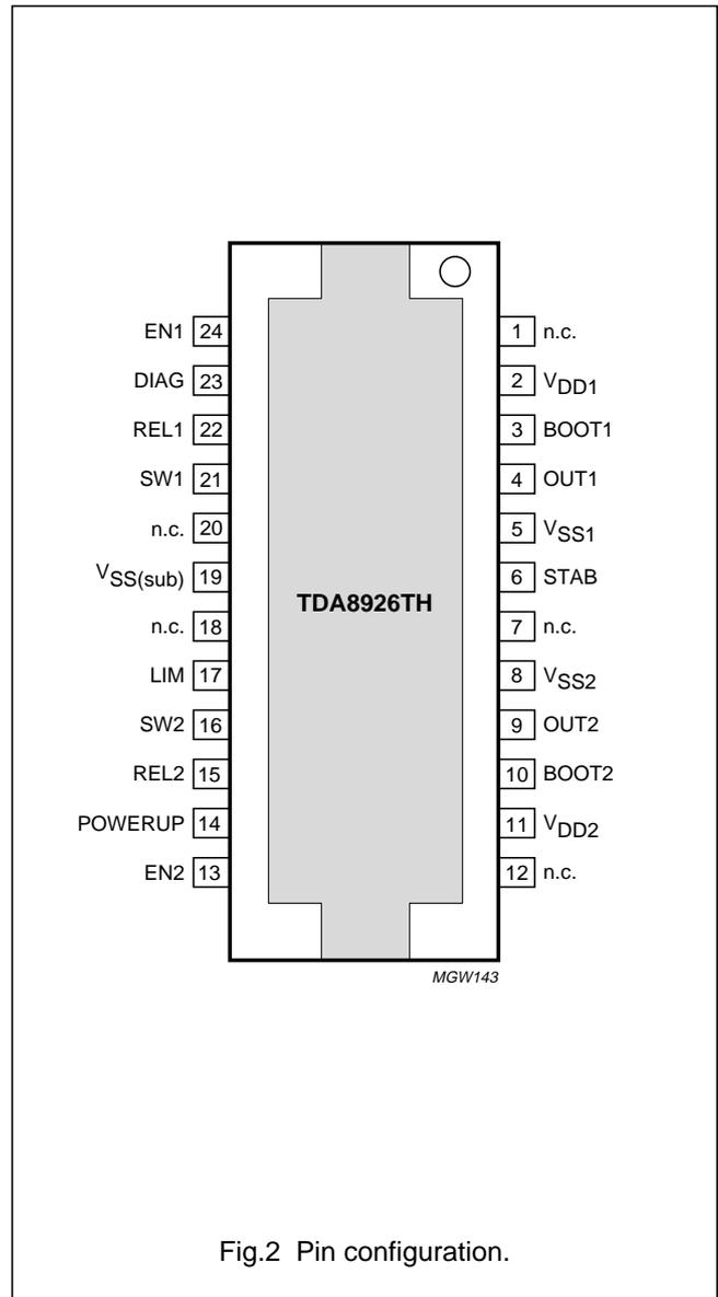
Fig.2 Pin configuration.
