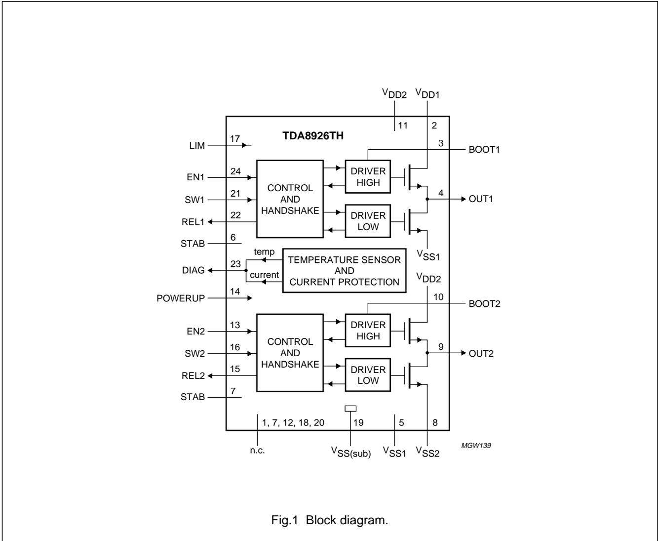
Fig.1 Block diagram.
