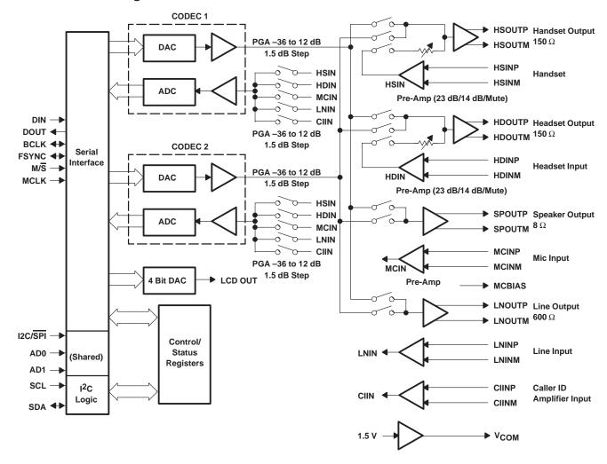
NOTE: Input and output analog signals are differential All switches are register controlled
