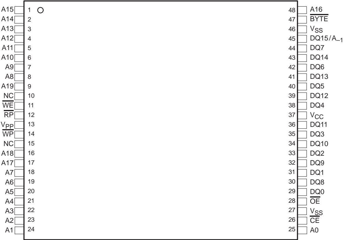
TMS28F1600T/B 48-PIN TSOP (DCD) (TOP VIEW)
