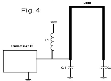
L1 just supplies the collector voltage for the output stage and is relatively large. For 314 to 433MHz 100 to 220nH is ok. C1 is set to give the desired load on the output stage. For the TH70211 and TH72031 transmitter, the load should be around 300 Ohms. C2 can then be used to tune the loop.
