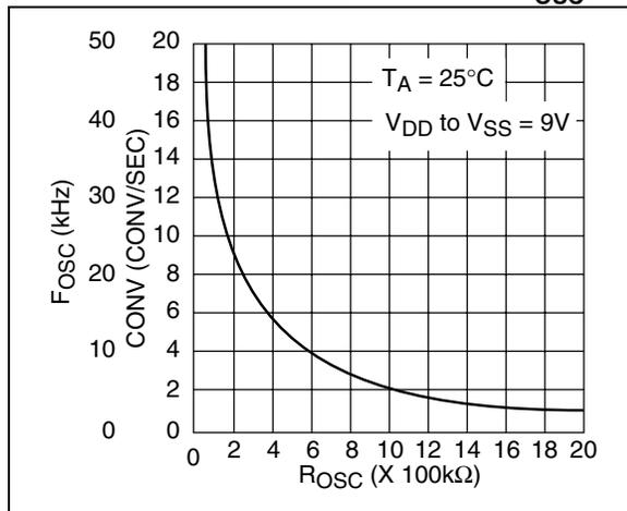
$F_{OSC}$  is divided by 32 to provide an internal system clock, FYSY. Each conversion requires 80 internal clock cycles. The internal system clock is divided by 8 to provide the LCD backplane drive frequency. The display flash rate during an input out-of-range signal is set by dividing FSYS by 320.
