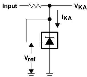
Figure 2. Test Circuit for  $V_{KA} = V_{ref}$
