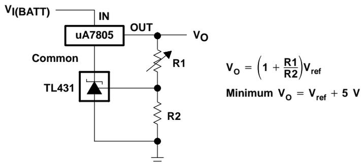
Figure 20. Output Control of a Three-Terminal Fixed Regulator
