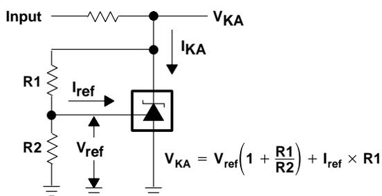
Figure 3. Test Circuit for  $V_{KA} > V_{ref}$
