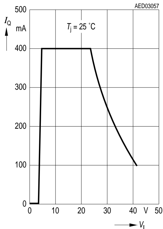
Output Current Limit I_Q versus Input Voltage V_I
