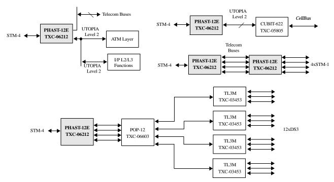
Note: Instead of connecting to the 2.488 Gbit/s PHY device, the serial interfaces of each PHAST-12E device can be connected to a 622 Mbit/s fiber optic transceiver for STS-12/STS-12c/STM-4/STM-4c operation. Alternatively, four 155 Mbit/s fiber optic transceivers can be connected to the line interfaces of each PHAST-12E device for quad STS-3c/STM-1 applications.
