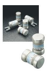
Littelfuse's TLS Series fuses are designed specifically for the protection of telecommunications equipment. TLS fuses have been engineered to operate up to 170 VDC to provide current limiting short circuit protection for cables and components found in the DC power distribution circuits of telecommunications systems. The TLS' compact design provides superior protection and high power density in an extremely compact package.
