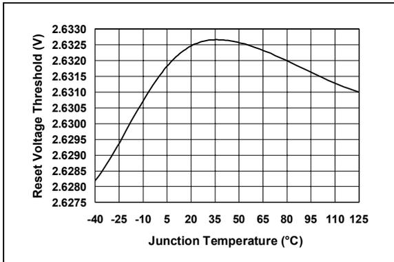
**FIGURE 2-8:** Reset Voltage Threshold vs. Junction Temperature.
