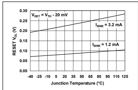
**FIGURE 2-17:** RESET Output Voltage Low
