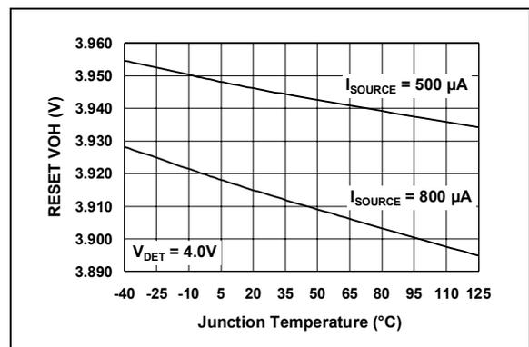
**FIGURE 2-18:** RESET Output Voltage High
