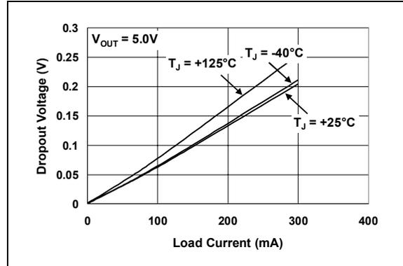
**FIGURE 2-10:** Dropout Voltage vs. Load Current (5.0V).
