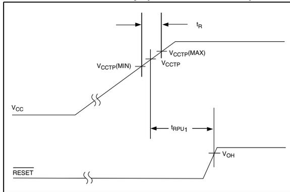
**FIGURE 3-2: Timing Diagram – Power Down (TC1275/TC1276)**
