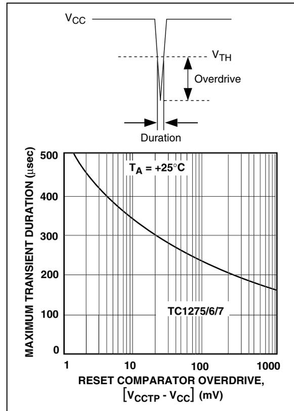
**FIGURE 3-6: ENSURING  $\overline{\text{RESET}}$  VALID TO  $V_{CC} = 0V$**
