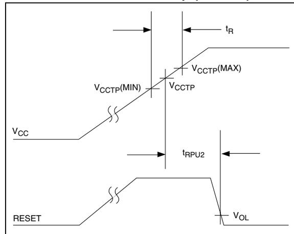
**FIGURE 3-4: Timing Diagram – Power Down (TC1277)**
