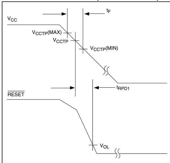
**FIGURE 3-3: Timing Diagram – Power Up (TC1277)**
