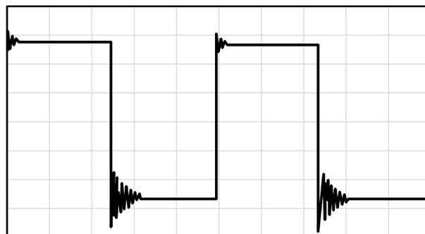
(b)  $C_L = 130 \text{ pF}$ ,  $R_L = \text{NO LOAD}$
