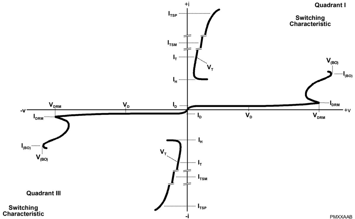
**Figure 1. VOLTAGE-CURRENT CHARACTERISTIC FOR T AND R TERMINALS
