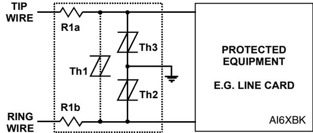
Figure 15. PROTECTION MODULE
