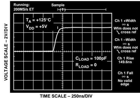
Figure 13. TMP04 Output Rise Time at +125°C
