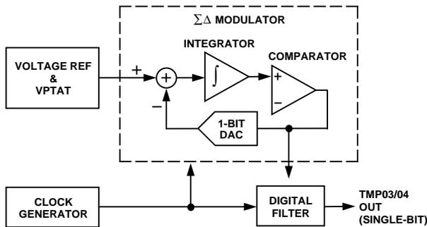
Figure 1. TMP03/TMP04 Block Diagram Showing First-Order Sigma-Delta Modulator
