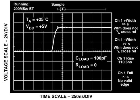
Figure 12. TMP04 Output Rise Time at +25°C
