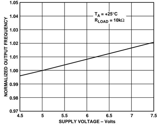
Figure 6. Normalized Output Frequency vs. Supply Voltage
