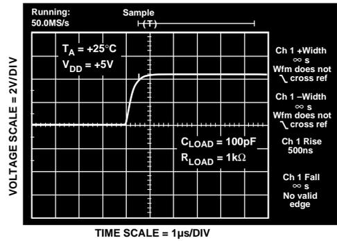
Figure 7. TMP03 Output Rise Time at +25°C
