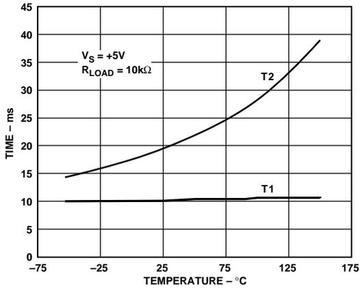
Figure 4. T1 and T2 Times vs. Temperature
