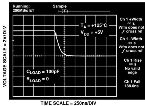
Figure 11. TMP04 Output Fall Time at +125°C
