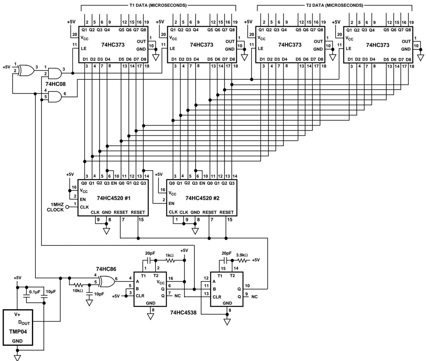
Figure 36. A Hardware Interface for the TMP04
