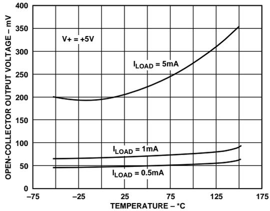
Figure 22. TMP03 Open-Collector Output Voltage vs. Temperature
