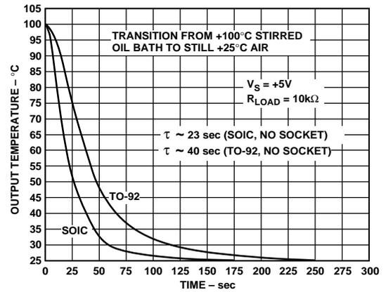
Figure 25. Thermal Response Time in Still Air
