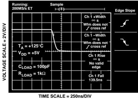
Figure 9. TMP03 Output Fall Time at +125°C
