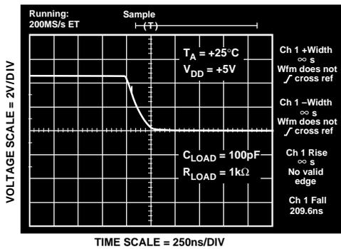
Figure 5. TMP03 Output Fall Time at +25°C
