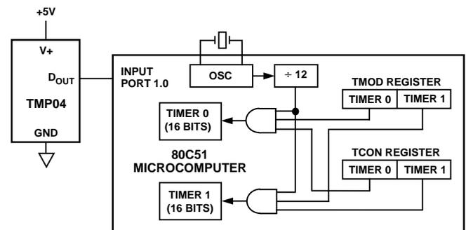
Figure 34. A TMP04 Interface to the 80C51 Microcomputer
