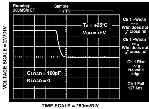
Figure 10. TMP04 Output Fall Time at +25°C
