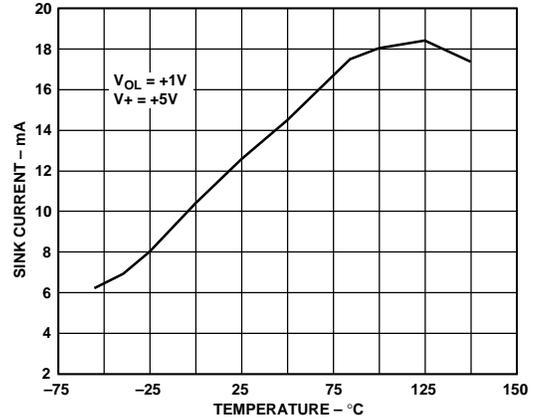
Figure 24. TMP03 Open-Collector Sink Current vs. Temperature
