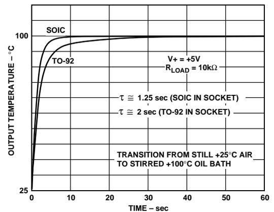
Figure 26. Thermal Response Time in Stirred Oil Bath
