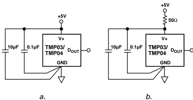
Figure 28. Recommended Supply Bypassing for the TMP03/TMP04
