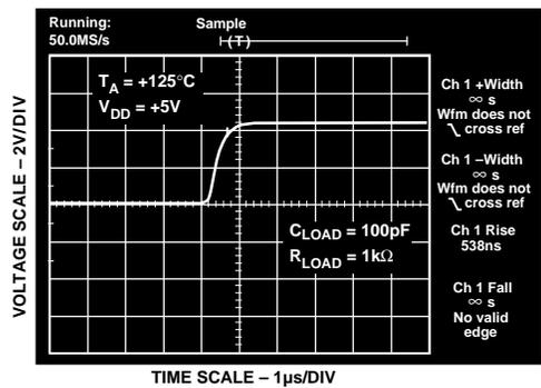
Figure 8. TMP03 Output Rise Time at +125°C
