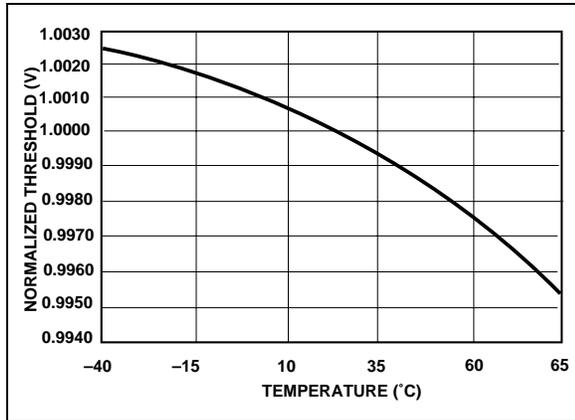
**FIGURE 3-7:** Normalized Reset Threshold vs. Temperature.
