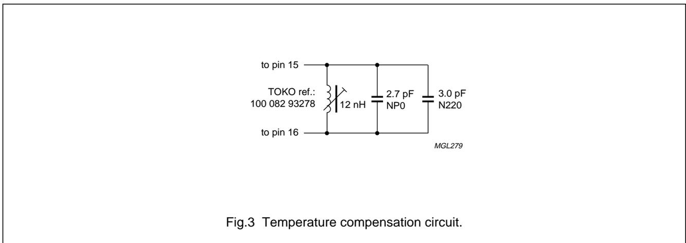
Fig.3 Temperature compensation circuit.
