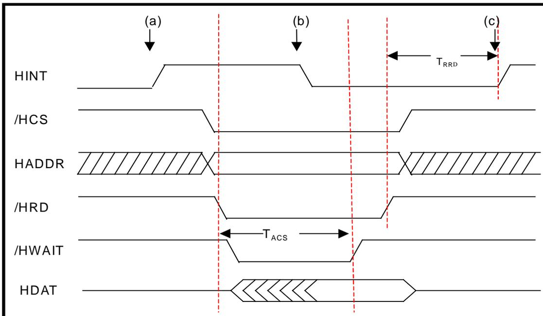
Fig. 7 Interrupt Operation
