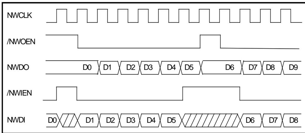
**Fig. 16 Network bit stream timing diagram (bit serial mode).**
