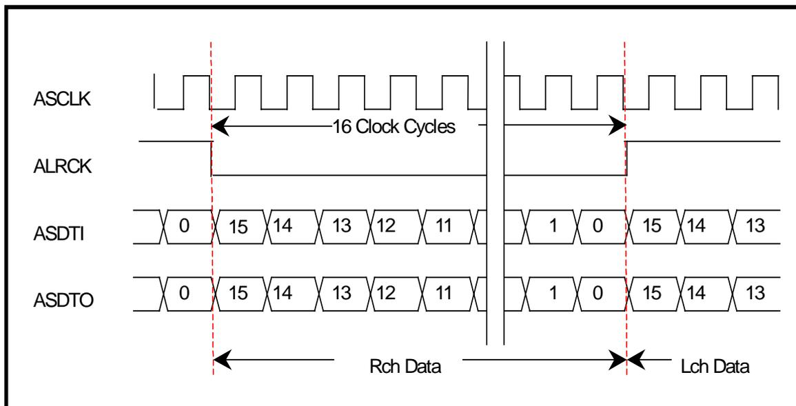
**Fig. 14 Audio ADC&DAC Interface (Master clock output mode).**
