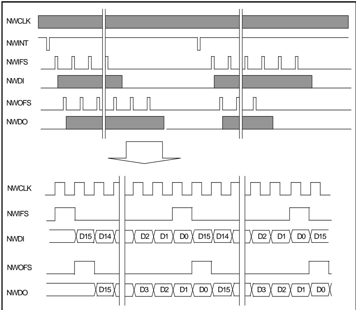
**Fig. 17 Network bit stream timing diagram (frame mode).**
