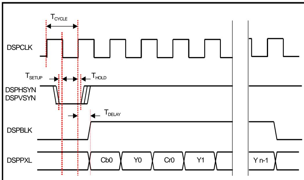
Fig. 12 Detail Timing Diagram of Display Interface.
