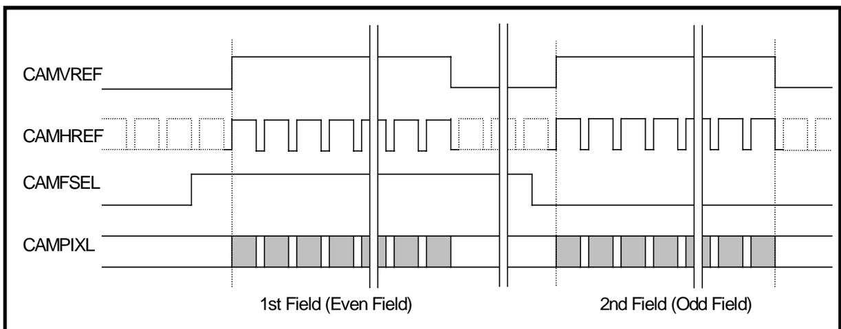
**Fig. 9 Field Based (NTSC) CAMVREF Timing Diagram**
