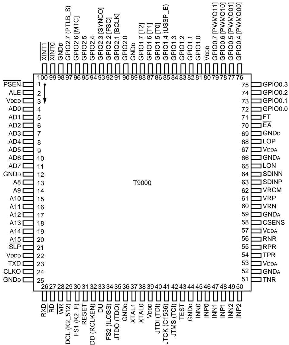
Note: Alternate pin functions, shown in parentheses (), are selected when the TEST pin is asserted.
