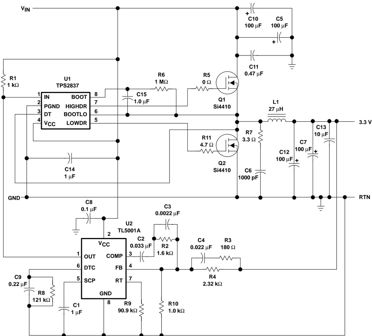
Figure 17. 3.3 V 3 A Synchronous-Buck Converter Circuit
