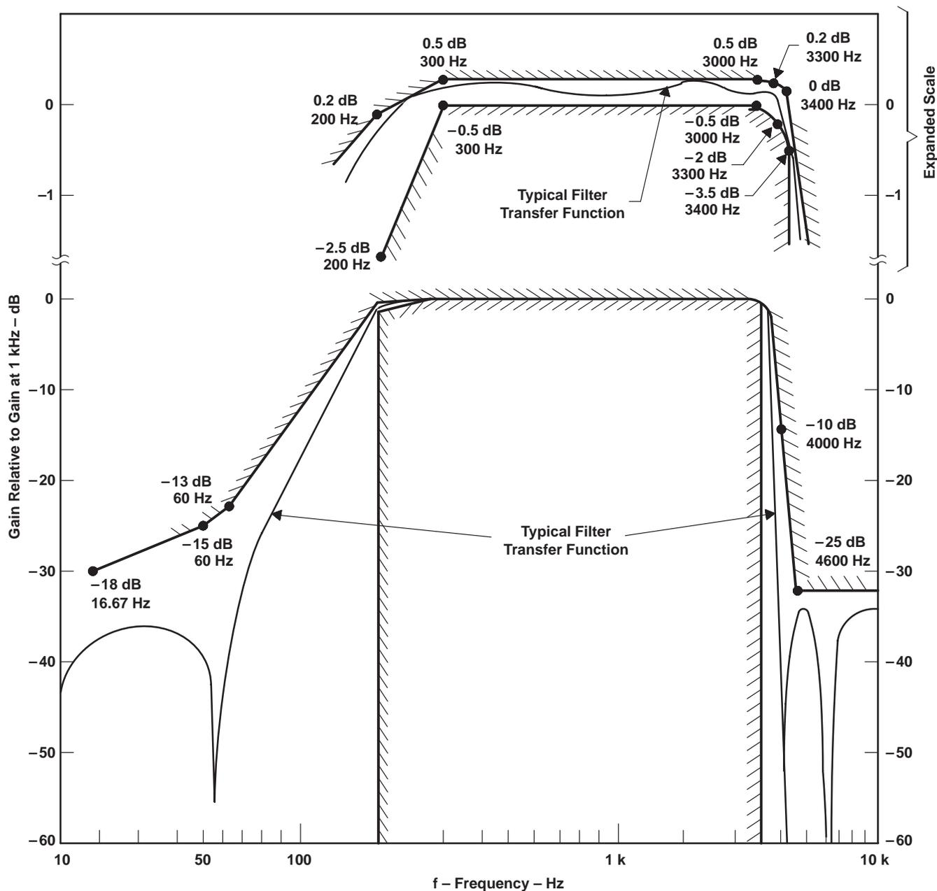
NOTE A: This is a typical transfer function of the receiver filter component.
