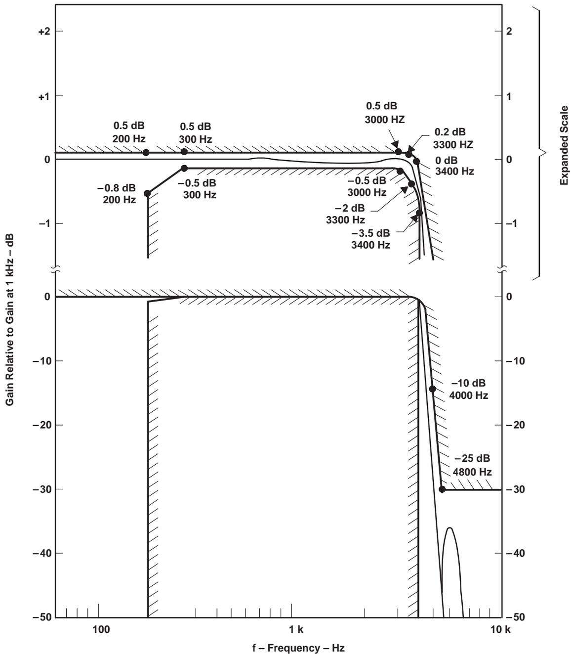
NOTE A: This is a typical transfer function of the receive filter component.
