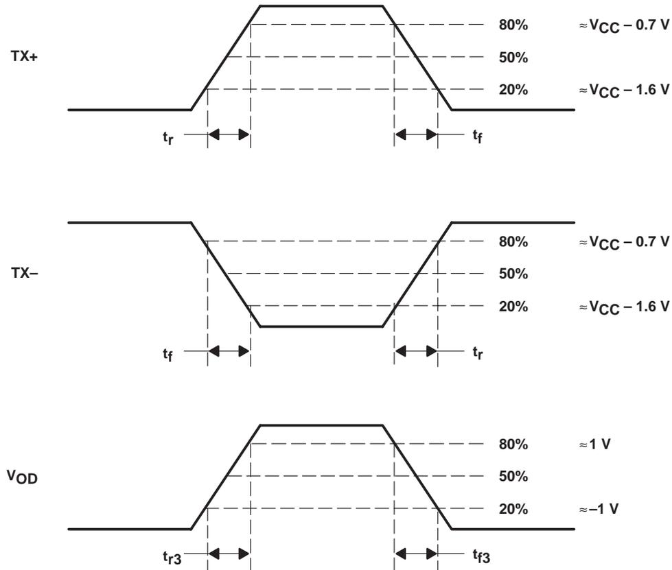
Figure 3. Differential and Common-Mode Output Voltage Definitions
