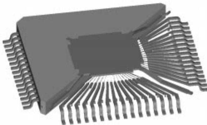
Figure 9. Heat-Spreader Design
