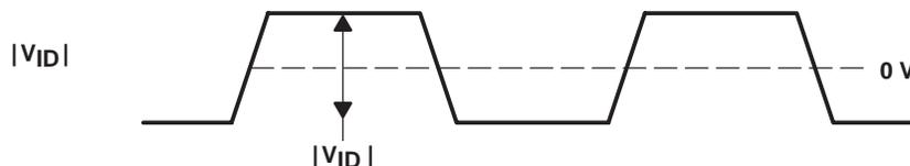
Figure 5. Differential Input Voltage (Peak-to-Peak) Timing Waveform
