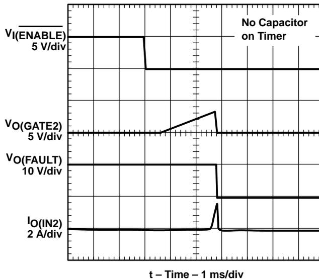
**Figure 10. Channel 2 – Enabled Into Short Circuit**
