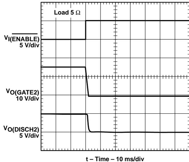
**Figure 4. Turnoff Voltage Transition of Channel 2**
