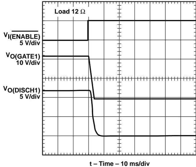
**Figure 2. Turnoff Voltage Transition of Channel 1**
