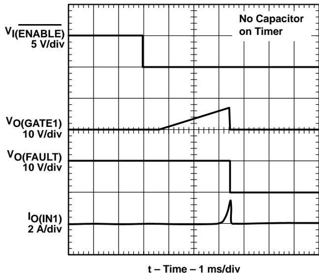
**Figure 9. Channel 1 – Enabled Into Short Circuit**
