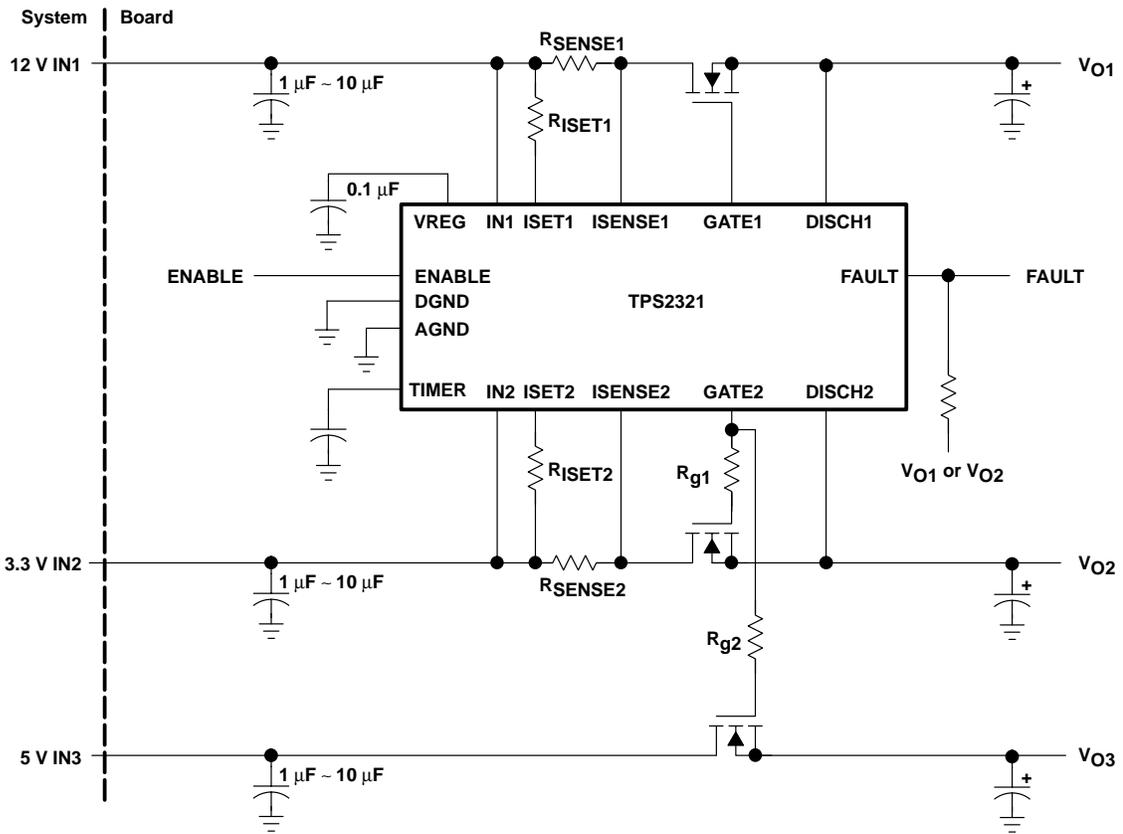
Figure 27. Three-Channel Application
