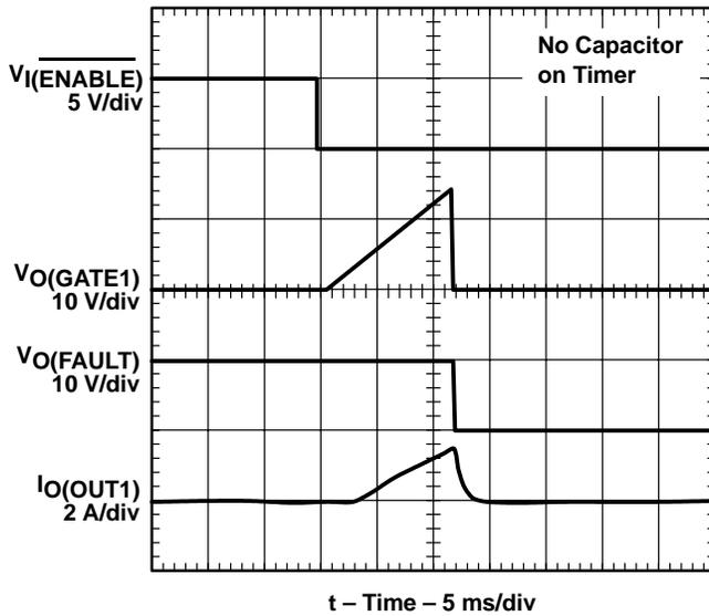
Figure 5. Channel 1 Overcurrent Response: Enabled Into Overcurrent Load
