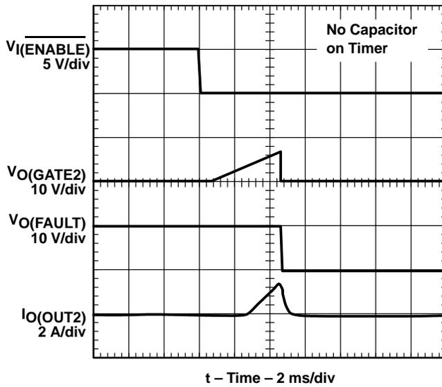
Figure 7. Channel 2 Overcurrent Response: Enabled Into Overcurrent Load
