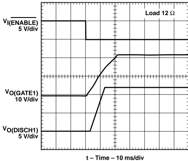
**Figure 1. Turnon Voltage Transition of Channel 1**
