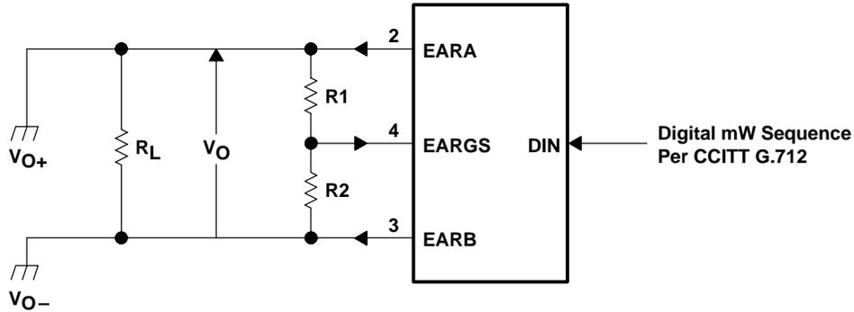
Figure 6. Gain-Setting Configuration
