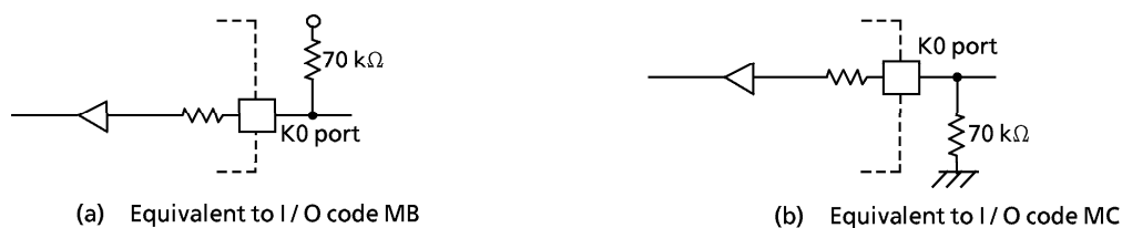
Figure 1-2. I / O code and external circuitry
