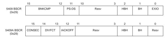
The CONSEC field of the 5409A BSCR is replaced functionally with the BNKCMP and PS-DS fields of the 5409 BSCR. The 5409A has a different external parallel interface from the 5409. The signals are identical but the timing waveform of signals is different. Refer to the 5409A data sheet (SPRS140) for more detail.
