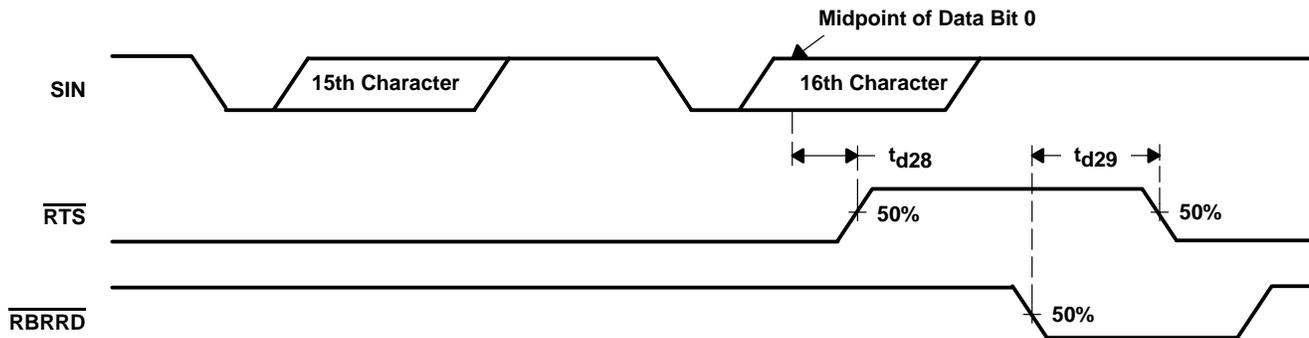
Figure 19. Auto-RTS Timing for RCV Threshold of 14 Waveforms
