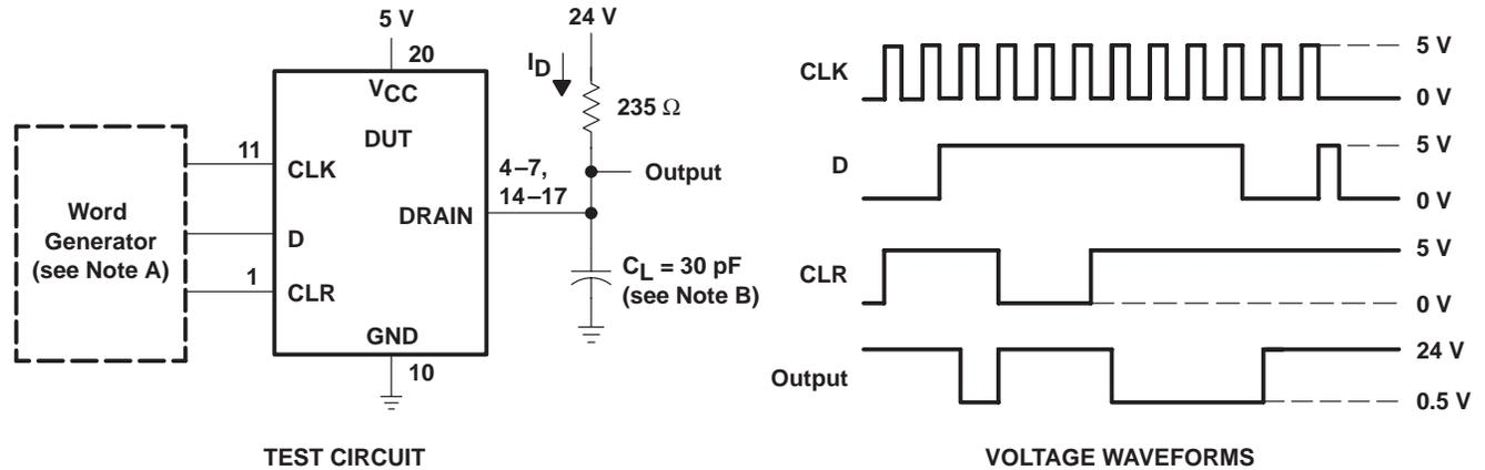
Figure 1. Resistive-Load Test Circuit and Voltage Waveforms
