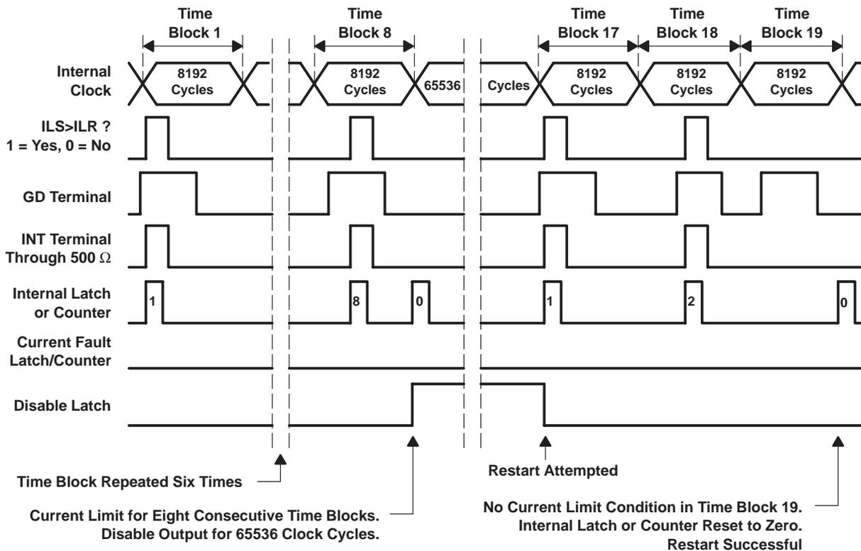
Figure 7. Current Fault Timing Diagram, Over-Current Limit Condition
