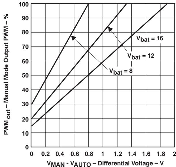
Figure 5. Manual Mode Input Signal vs. Output PWM
