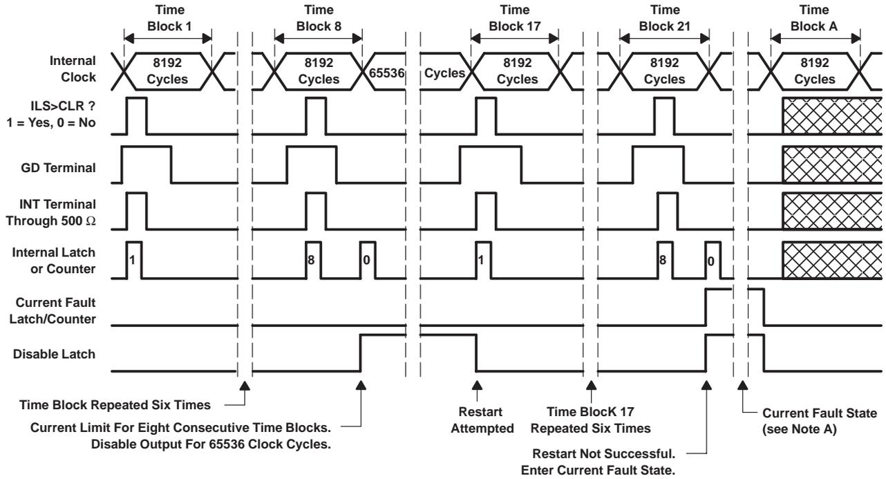
NOTE A: The integrated circuit remains in this state until cycled through the sleep state into the run state. Timing resumes as shown in time block A at right.
