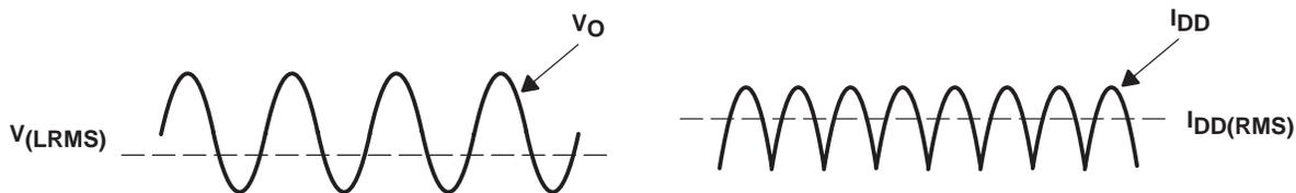
Figure 36. Voltage and Current Waveforms for BTL Amplifiers
