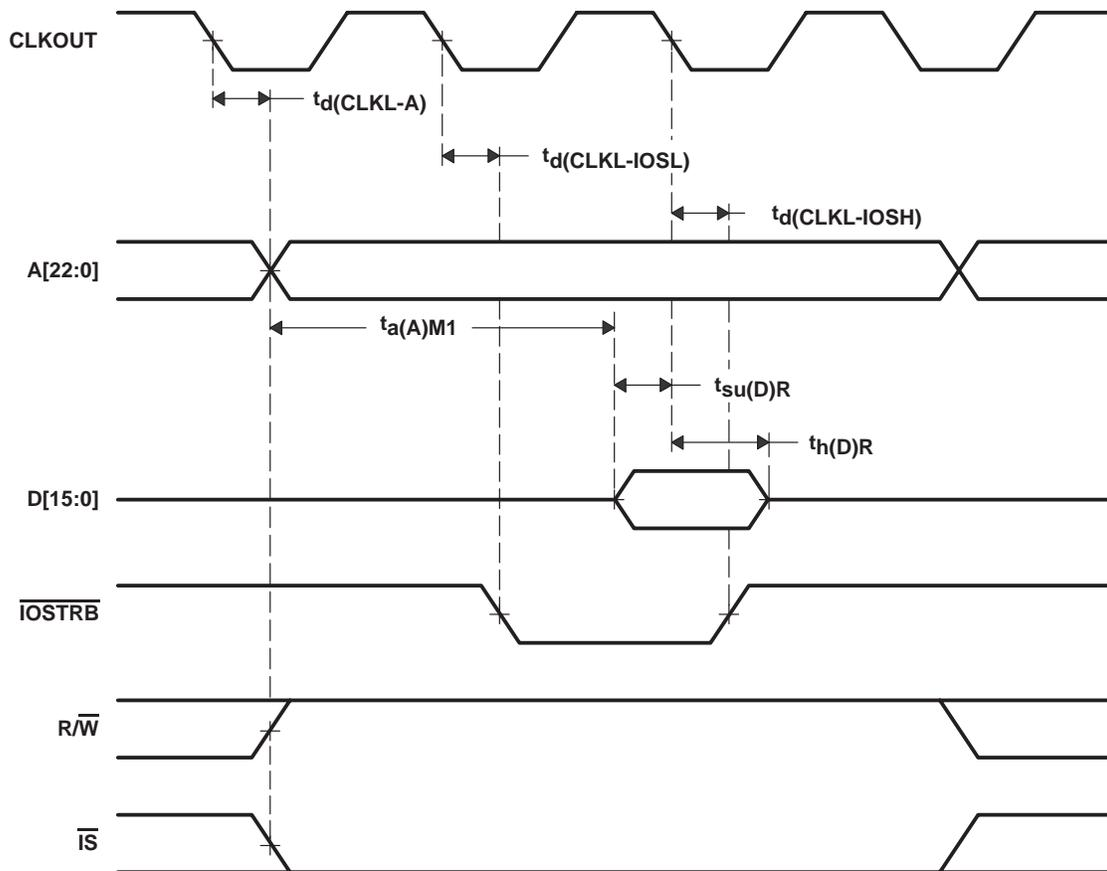
Figure 4–8. Parallel I/O Port Read ( $\overline{\text{IOSTRB}} = 0$ )
