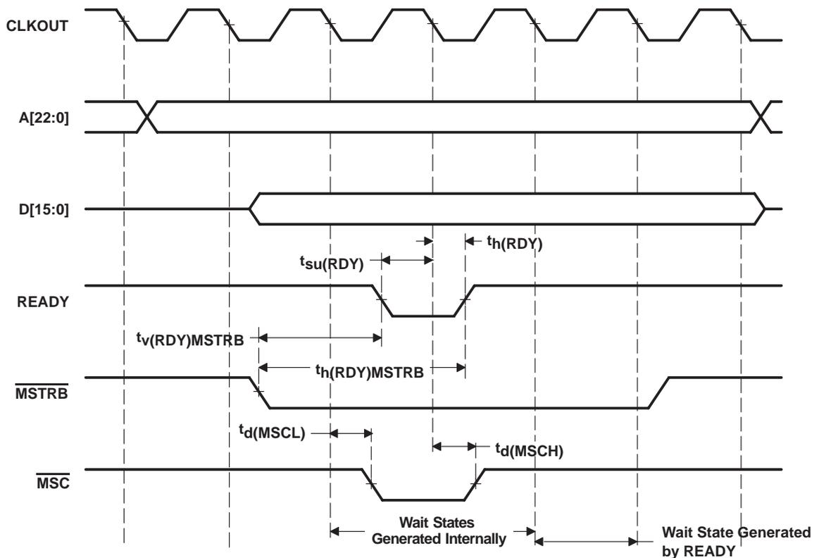
Figure 4–11. Memory Write With Externally Generated Wait States
