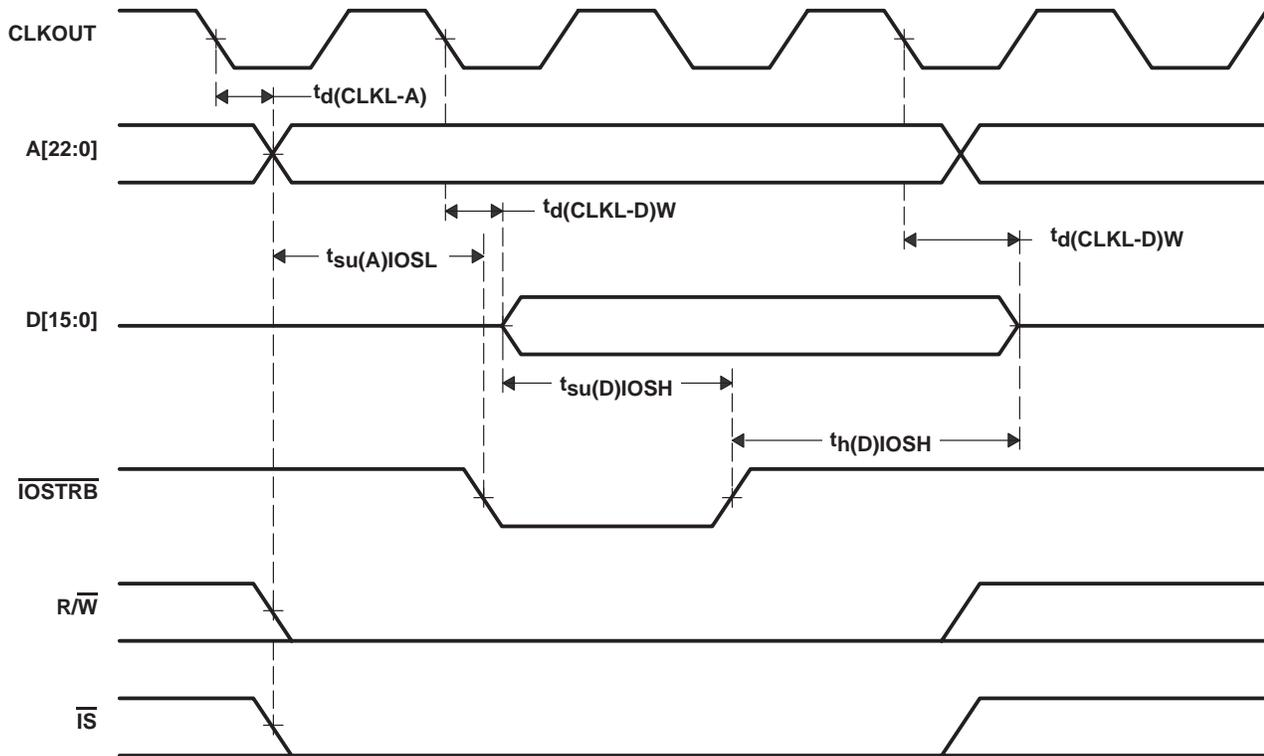
Figure 4–9. Parallel I/O Port Write ( $\overline{\text{IOSTRB}} = 0$ )
