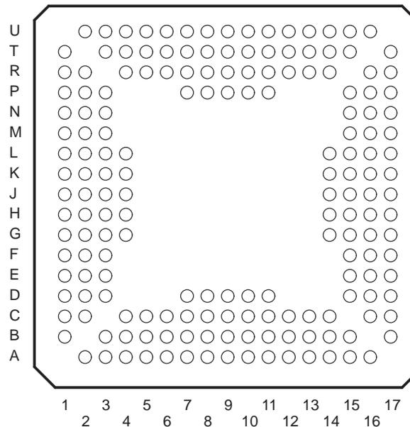
Figure 1–1. 176-Ball GGW MicroStar BGA™ (Bottom View)
