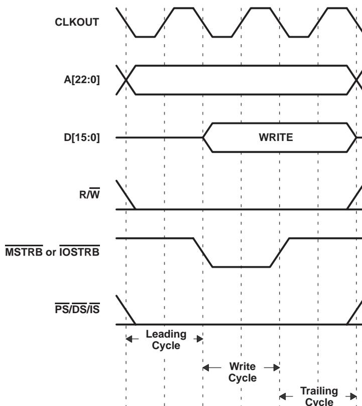
**Figure 2–11. Memory Write and I/O Write Bus Sequence**
