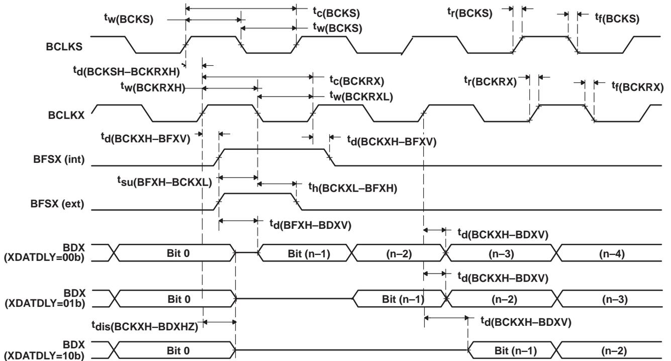
Figure 4–22. McBSP Transmit Timings
