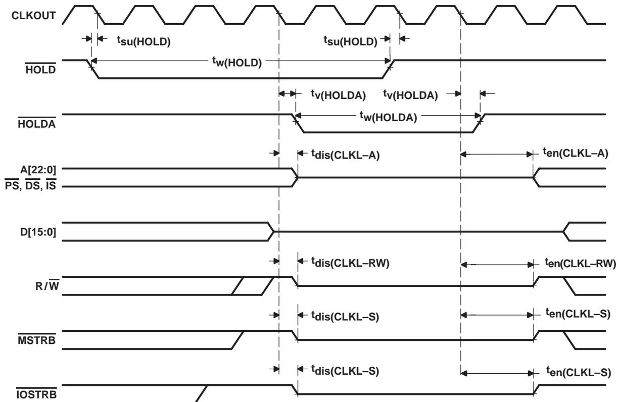
**Figure 4–14.  $\overline{\text{HOLD}}$  and  $\overline{\text{HOLDA}}$  Timings (HM = 1)**
