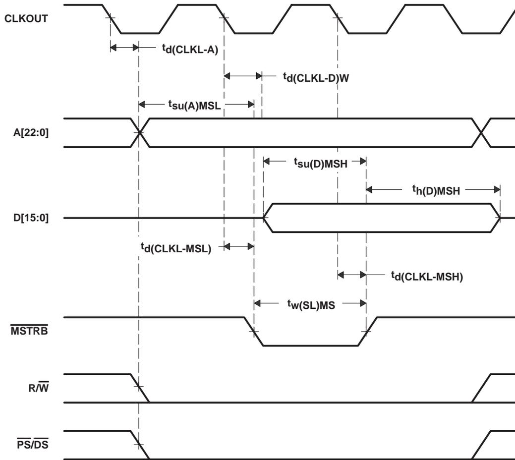
Figure 4–7. Memory Write ( $\overline{\text{MSTRB}} = 0$ )
