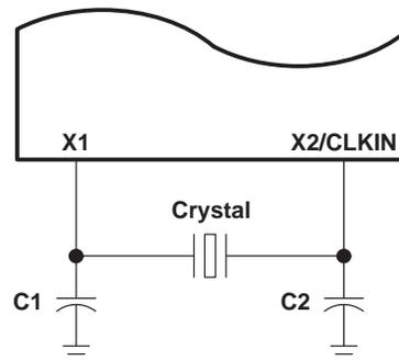
Figure 4–2. Internal Divide-by-Two Clock Option With External Crystal
