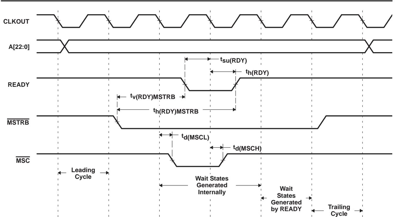
Figure 4–10. Memory Read With Externally Generated Wait States
