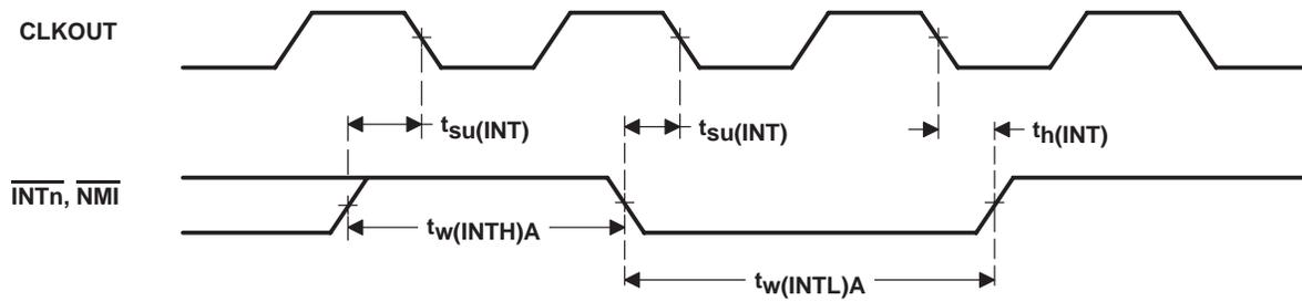
Figure 4-16. Interrupt Timing
