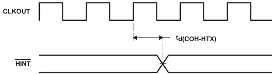
Figure 4-30.  $\overline{\text{HINT}}$  Timing
