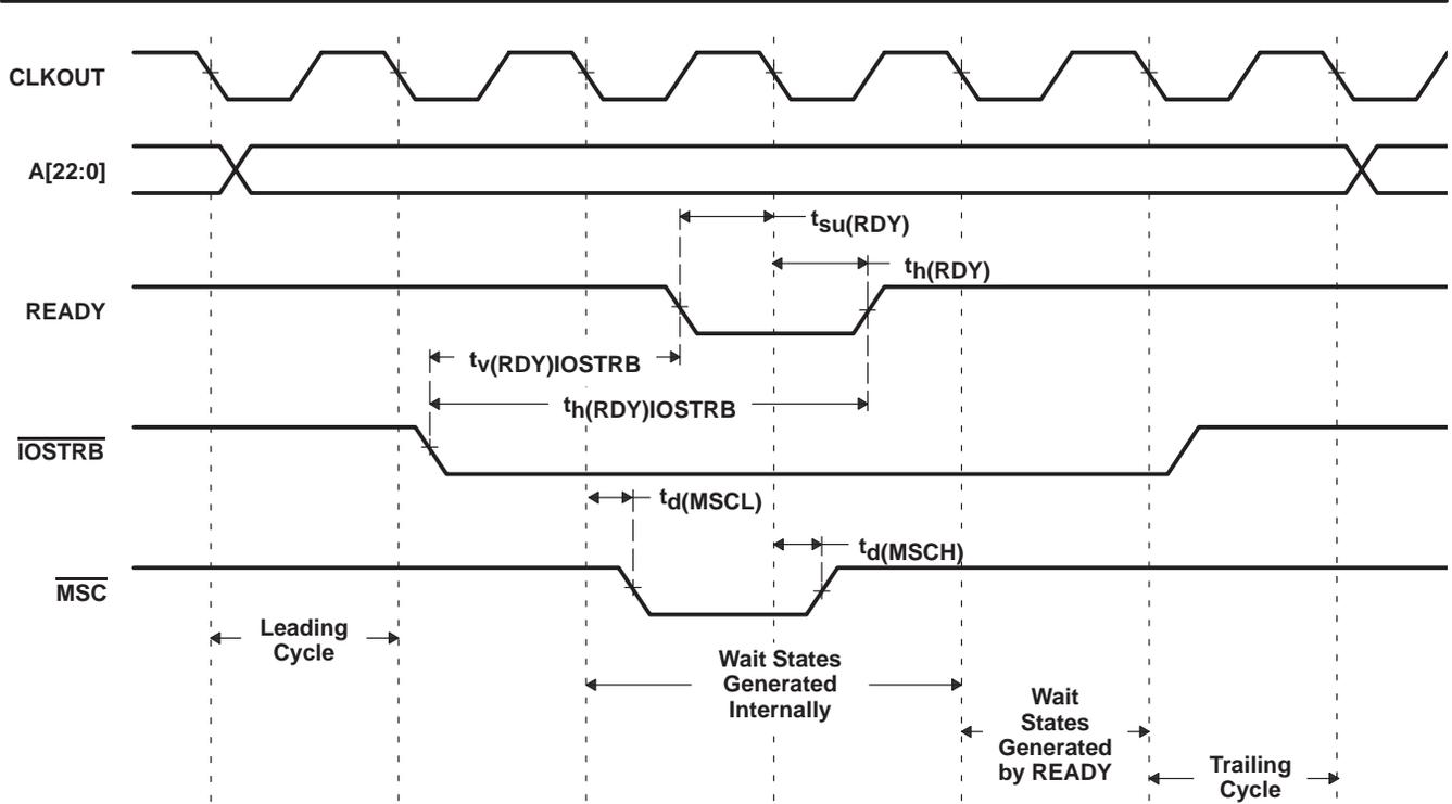
Figure 4–12. I/O Read With Externally Generated Wait States
