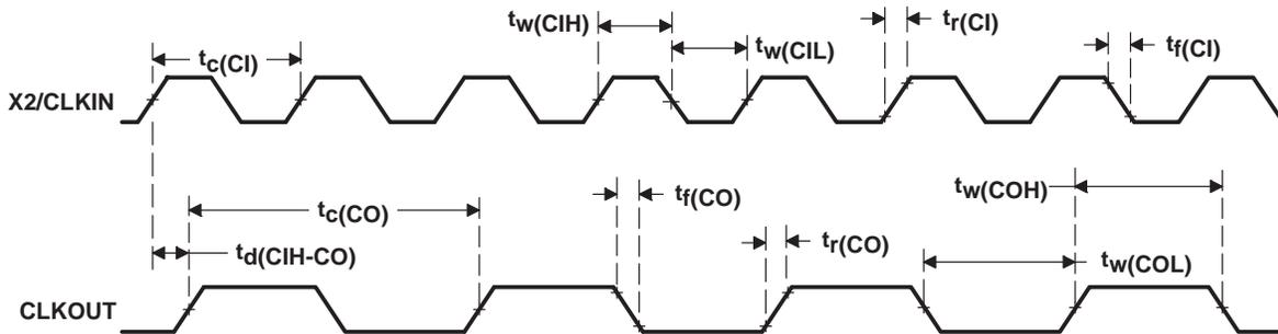
NOTE A: The CLKOUT timing in this diagram assumes the CLKOUT divide factor (DIVFCT field in the BSCR) is configured as 00 (CLKOUT not divided). DIVFCT is configured as CLKOUT divided-by-4 mode following reset.
