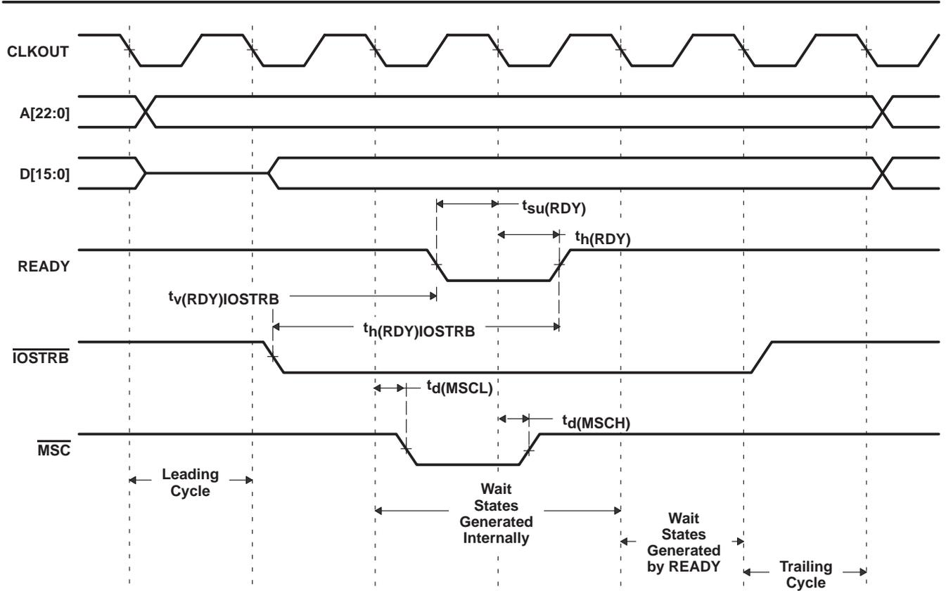
Figure 4–13. I/O Write With Externally Generated Wait States
