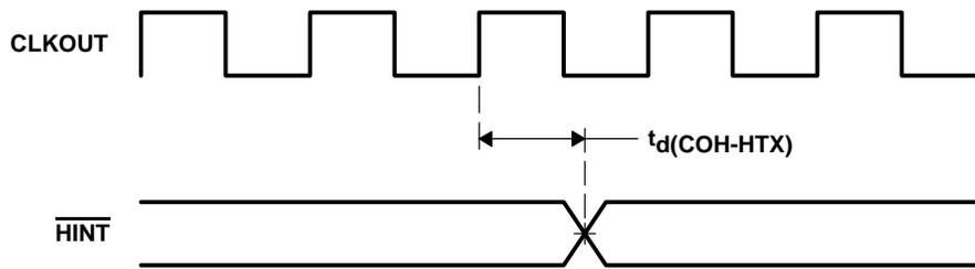
Figure 4-30.  $\overline{\text{HINT}}$  Timing
