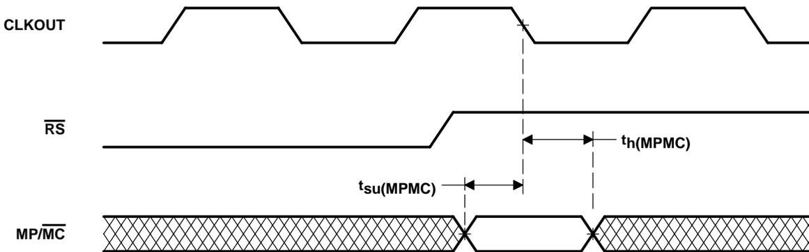
Figure 4–16.  $\overline{\text{MP/MC}}$  Timing
