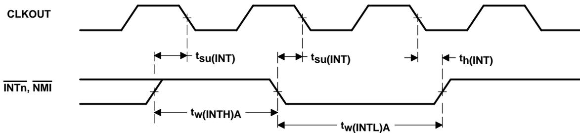
Figure 4–15. Interrupt Timing
