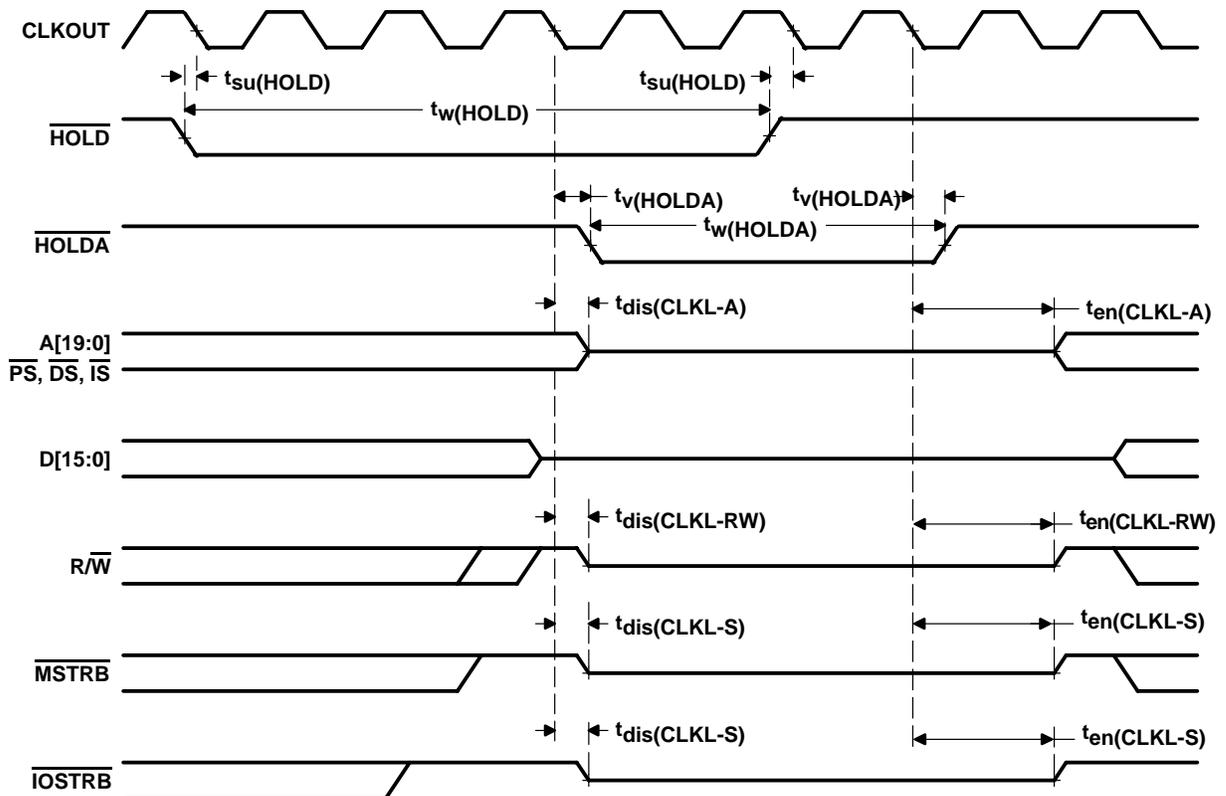
Figure 4–13.  $\overline{\text{HOLD}}$  and  $\overline{\text{HOLDA}}$  Timings (HM = 1)
