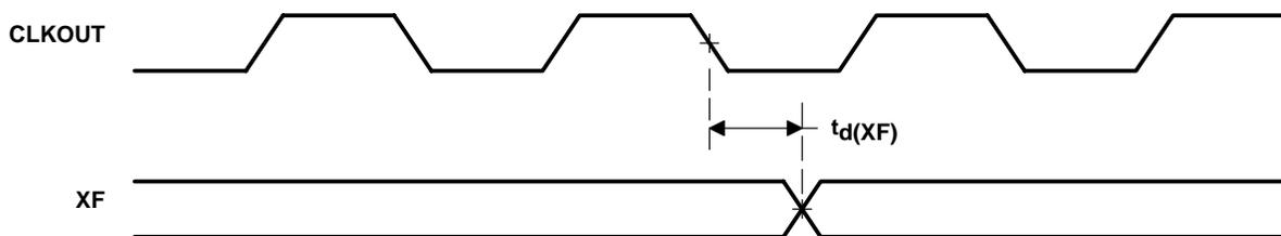
**Figure 4–18. XF Timing**
