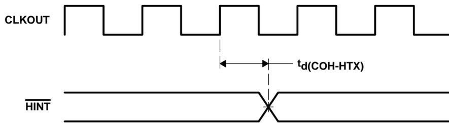
Figure 4-29.  $\overline{\text{HINT}}$  Timing
